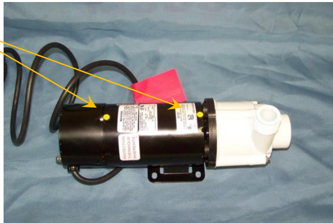
Figure 8: Oil hole locations on the FilterMax pump
