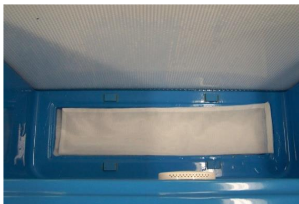
Figure 4: showing the Velcro bag, filled with carbon on top of the first media pad.
